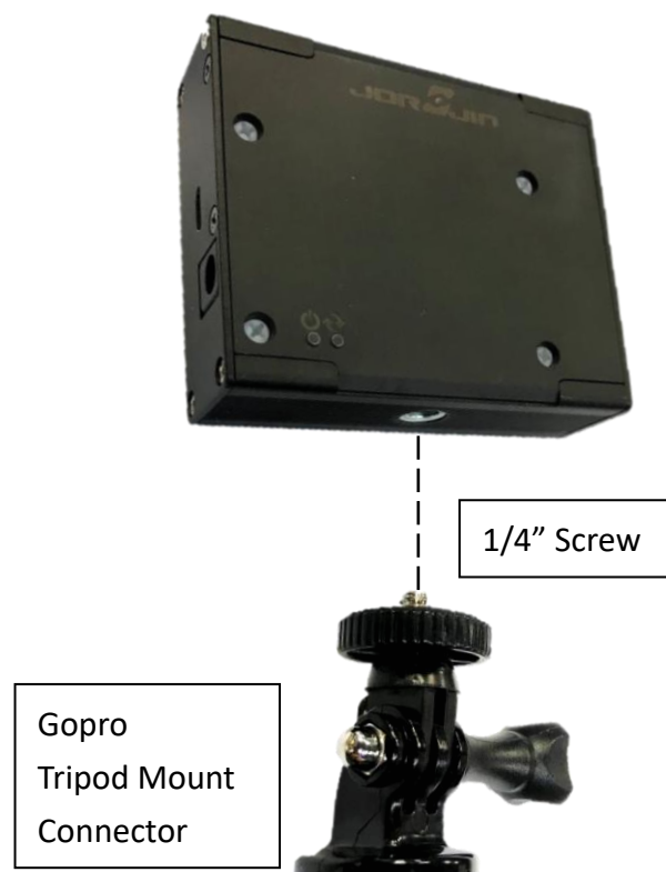
Figure 2-8. Gopro Mount explosion drawing
